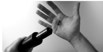
Separate piston from the base of the mechanism, exposing the adjust screw.
