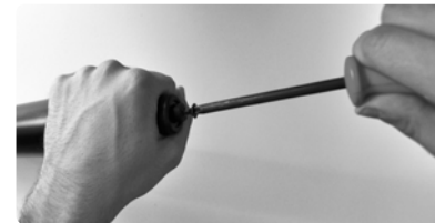
Regulate inward screw 1 and 2 mm. Reassemble and check.
