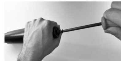
Regulate the screw out 1 to 2 mm. Reassemble and check.
