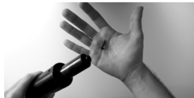
Separe piston from the base of the mechanism, exposing the adjust screw.
